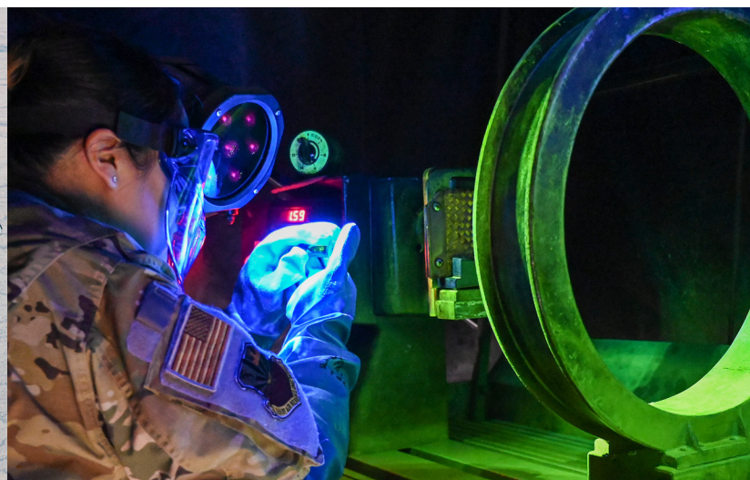
Staff Sgt. Erica Stanton, 161st non-destructive inspection technician, inspects a batch of aircraft bolts in the NDI Lab at Goldwater Air National Guard Base Photo by Tech. Sgt. Dillon Davis
