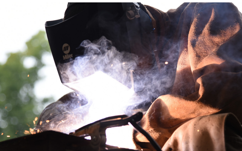
Airman 1st Class Dylan Pattee, 161st Civil Engineer Squadron, structures apprentice, utilizes a metal inert gas welder during training in New London, N.C., Aug. 3, 2021. Photo by Master Sgt. Michael Matkin
