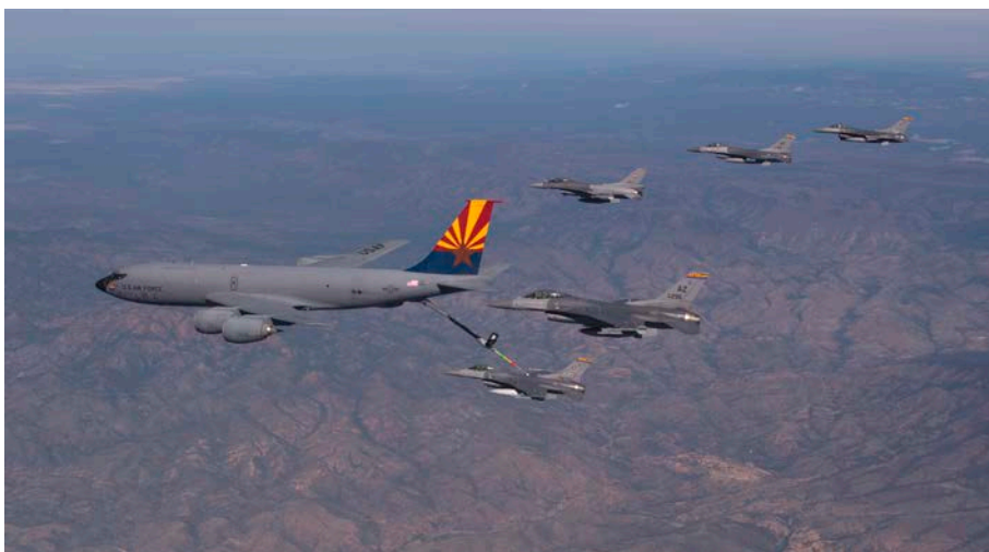
A 161 st Air Refueling Wing KC-135R Stratotanker refuels F-16 Fighting Falcons from the 162 nd Wing based in Tucson, April 8, 2015. (Photo by Master Sgt. Jeffrey Allen)
