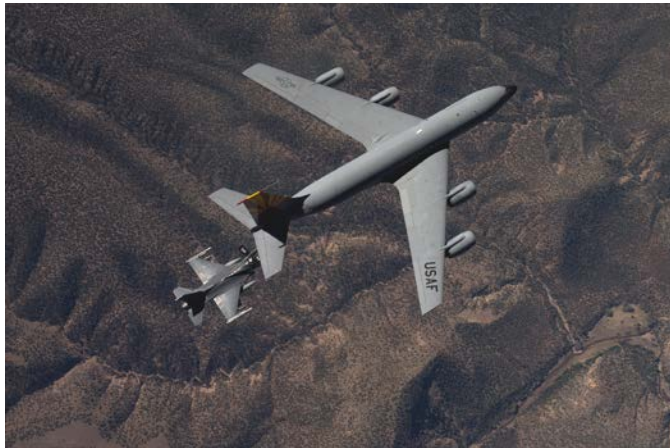
A 161 st Air Refueling Wing KC-135R Stratotanker refuels an F-16 Fighting Falcon from the 162 nd Wing, April 8, 2015. (Photo by Master Sgt. Jeffrey Allen)
