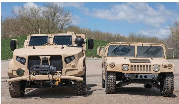
The space requirements for Readiness Centers are only going to increase. For example, compare the size of the Joint Light Tactical Vehicle (left) that is replacing the HMMWVs (right), which entered Army service in 1984. Oshkosh Photo
