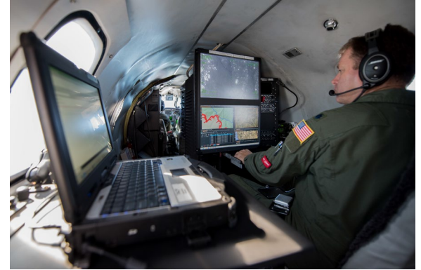
RC-26 mission system operator maps the Chetco Bar fire in southern Oregon using the RC-26s camera Sept. 2, 2017, Brookings, Oregon. Before the RC-26 were used to map fires, firefighters would drive out along the fire line to map out its location, taking hours to complete, putting the firefighters in danger and causing information to be 25-36 hours out of date. (USAF/Senior Airman Sean Campbell)
